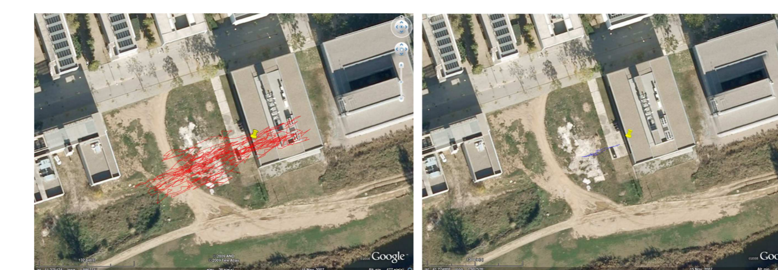
FIGURE 8: 120s static receiver position evolution for LMS (left) and Kalman (right) Solver
